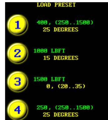
Figure 5.17-3: Pre-sets 1 and 4 with Torque Limits in Brackets
