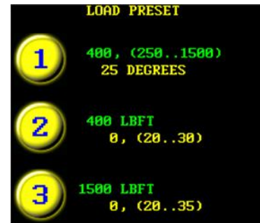
Figure 5.18-3: Pre-sets 2 and 3 with Angle Limits in Brackets
