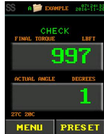
Figure 7.2-6: Torque Checked Cycle
