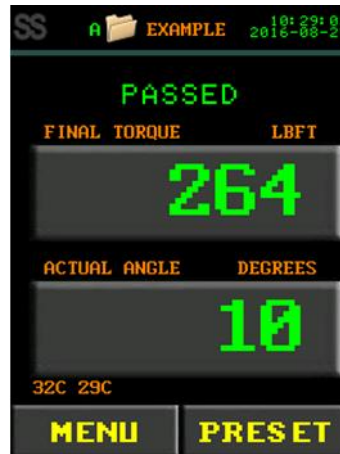
Figure 7.3-2: Passed Angle Cycle
