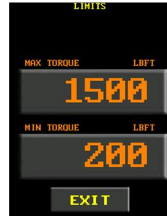
Figure 5.17-2: Set Min and Max Torque Limits
