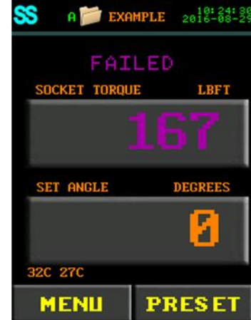
Figure 7.2-4: Failed Torque Cycle with Smart Socket Result
