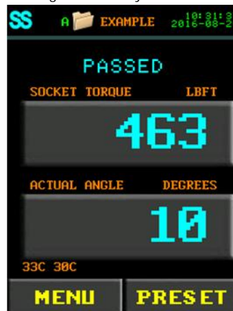
Figure 7.4-4: Passed Torque and Angle with Smart Socket
