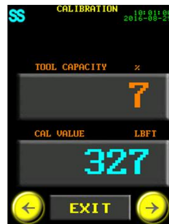
Figure 6-4: Calibration Value from Sensor/Smart Socket
