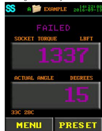
Figure 7.4-5: Failed Torque and Angle with Smart Socket
