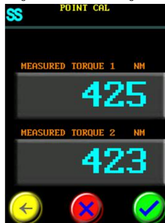
Figure 5.15-4: Point Calibration Screen
