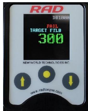
Figure 4.2-2: Failed Torque Cycle
