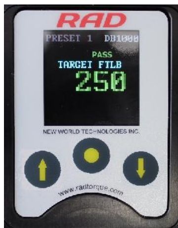
Figure 4.2-1: Passed Torque Cycle
