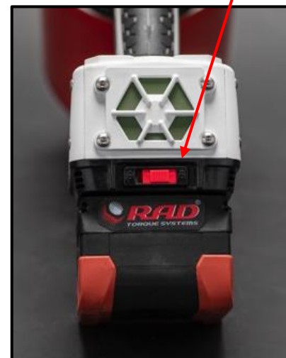
Figure 2.3.1-1: Battery Release and Lock Out
