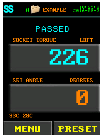
Figure 7.2-3: Passed Torque Cycle with Smart Socket Result
