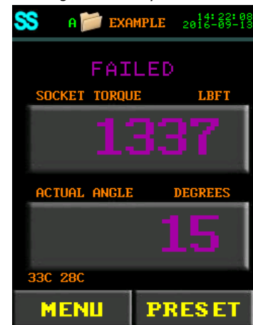
Figure 7.4-5: Failed Torque and Angle with Smart Socket
