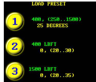
Figure 5.17-3: Presets 2 and 3 with Angle Limits in Brackets
