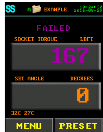
Figure 7.2-4: Failed Torque Cycle with Smart Socket Result
