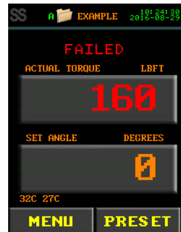
Figure 7.2-2: Failed Torque Cycle
