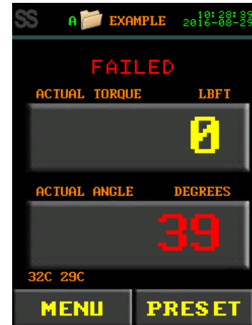
Figure 7.3-3: Failed Angle Cycle
