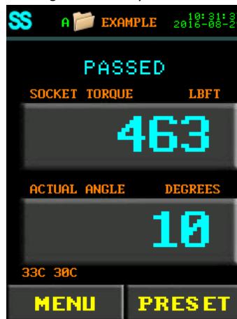
Figure 7.4-4: Passed Torque and Angle with Smart Socket
