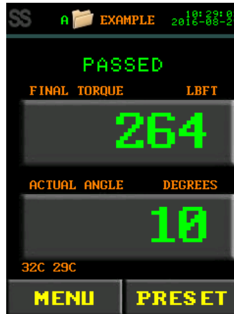
Figure 7.3-2: Passed Angle Cycle
