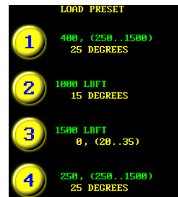
Figure 5.16-3: Presets 1 and 4 with Torque Limits in Brackets
