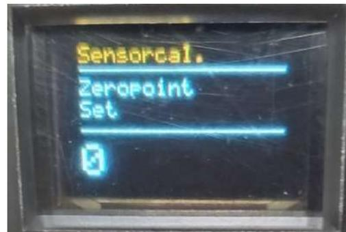
Figure 5.4-1: Sensorcal – Zero Point Setting
