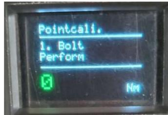
Figure 3.3.6-2: Bolt 1 Torquing Screen
