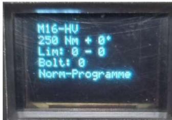
Figure 3.2.3-3: HV-Preset Details Screen
