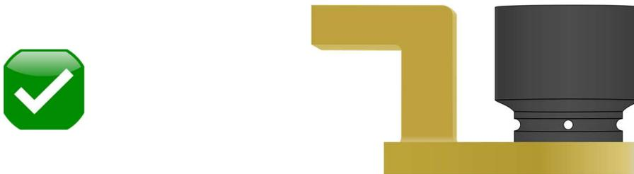
The height of the socket cannot be shorter or longer than the height of the Reaction Arm.
