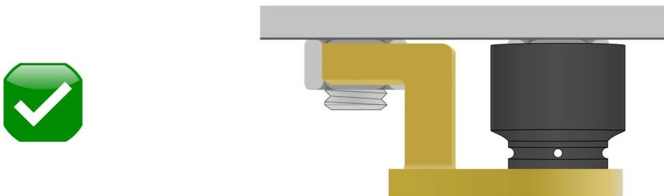
The length of the foot cannot be shorter or longer than the reaction point.
