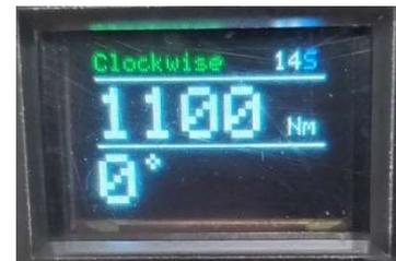
Figure 4.2-1: Torque Select Mode
