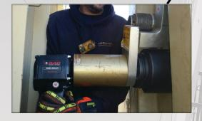
RAD 85GX used to install Wrist Pin
