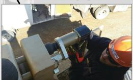
RAD 25GX used to install Crank Bolts
