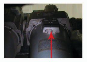
Bottom Side Filling: Pull the release lever downward and twist the entire bowl to the right or left while pulling downward. Remove the bowl and fill with lubricant.
