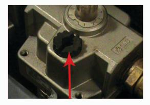
**Top Side Filling:** Remove the black fill plug and fill with lubricant.
